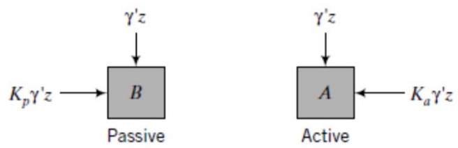
FIGURE 15.2 Stresses on soil elements in front of and behind a retaining wall.
